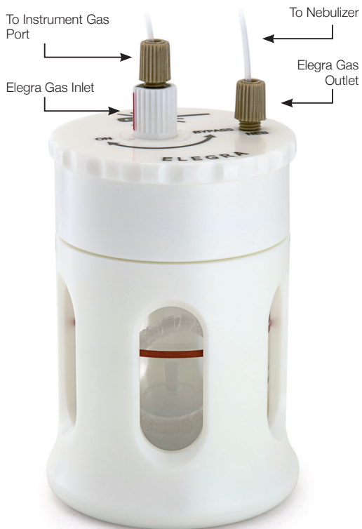
Figure 2. Elegra Argon Humidifier Installation (Agilent 5100 ICP-OES) Figure 2a
