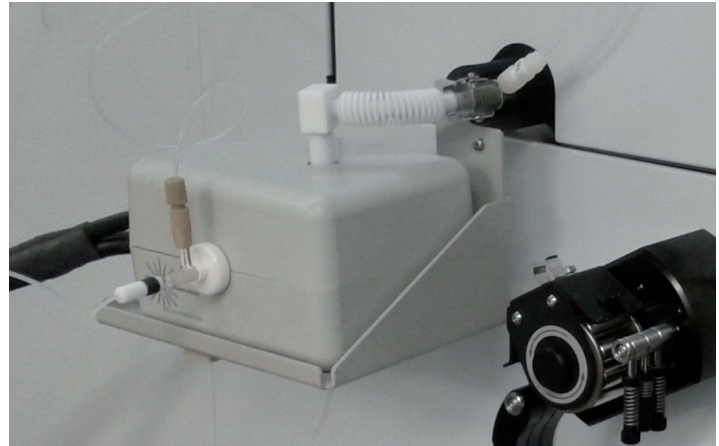
Figure 4: PCC Spray Chamber mounted on an Agilent 7700 ICP-MS
