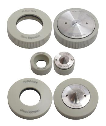
When cleaning cones which have a screw thread, it is important that the thread does not come in contact with any corrosive solution. If the thread gets corroded, the cone may not seal correctly or it may bond to the base and be difficult to remove. And with Pt cones, the thread is likely to wear out before the Pt insert.
