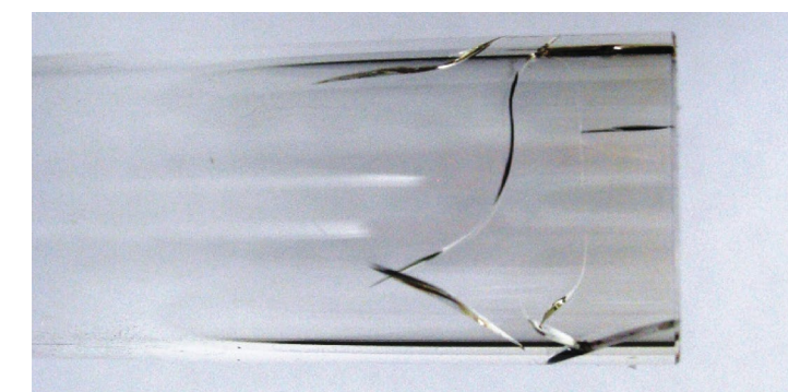
Quartz torches often crack upon cooling due to thermal shock when running organic solvents.
