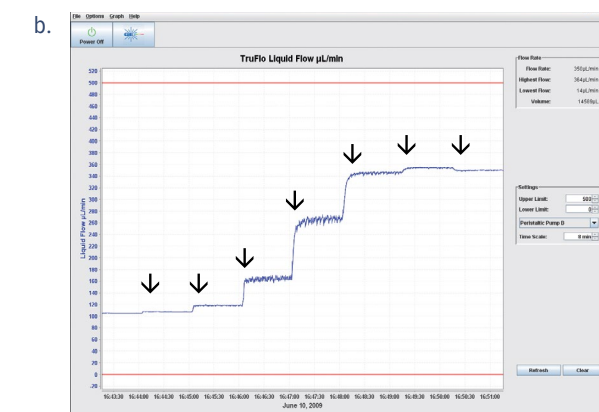
Adjusting pump tension
