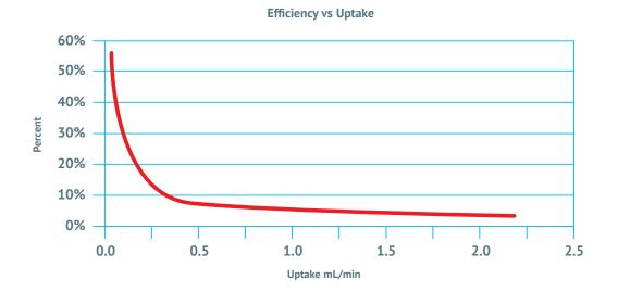
The 50ul/min nebulizer has 50% efficiency and therefore injects 25ul/min into the plasma. On the other hand, the standard 2ml/min nebulizer has 2% efficiency, resulting in 40ul/min of sample injected into the plasma. This means that the MicroMist nebulizer can reduce sample consumption by a factor of 40 and yet the sensitivity is reduced by less than a factor of two.
