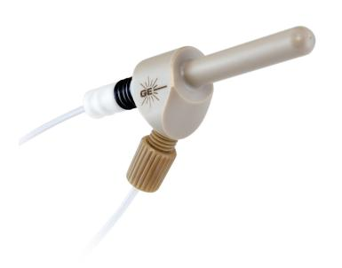
The DuraMist™ is a HF-resistant nebulizer, providing excellent sensitivity and precision at an affordable price. The DuraMist is a concentric, self-aspirating nebulizer and is compatible with all ICP models. And its ability to run samples with up to 30% total dissolved solids without blockage make it effectively a universal nebulizer.
