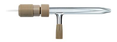
Glass Expansion is the only manufacturer that takes thick walled constantbore tubing and machines the outside to a uniform aerodynamic shape. This guarantees a uniform sample channel, assuring tolerance to high matrix samples and perfect reproducibility.
