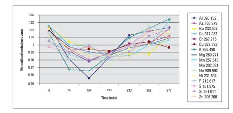
Figure 10. Long-term stability of 20 analyte wavelengths with the IsoMist at 25C.
