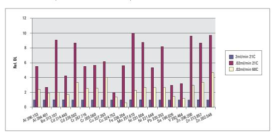
Figure 8. Effect of spray chamber temperature on oxide ratio<sup>2</sup>.
