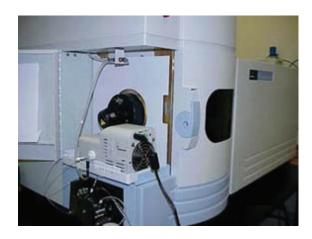
Figure 3. IsoMist mounted on the Optima 2100DV.
