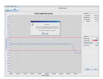
You receive a warning on the screen, as well as an audible alarm, if the sample flow moves outside the acceptable range.
