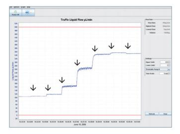
The realtime flow display enables you to optimise the pressure on the peristaltic pump tubing. The clamp was tightened by a half turn at each arrow.
